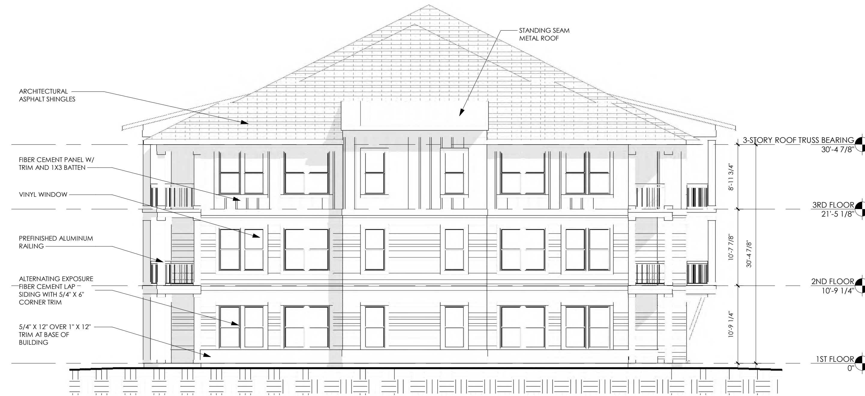
2 BLDG TYPE D - SIDE 2 ELEVATION 1/8" = 1'-0"
