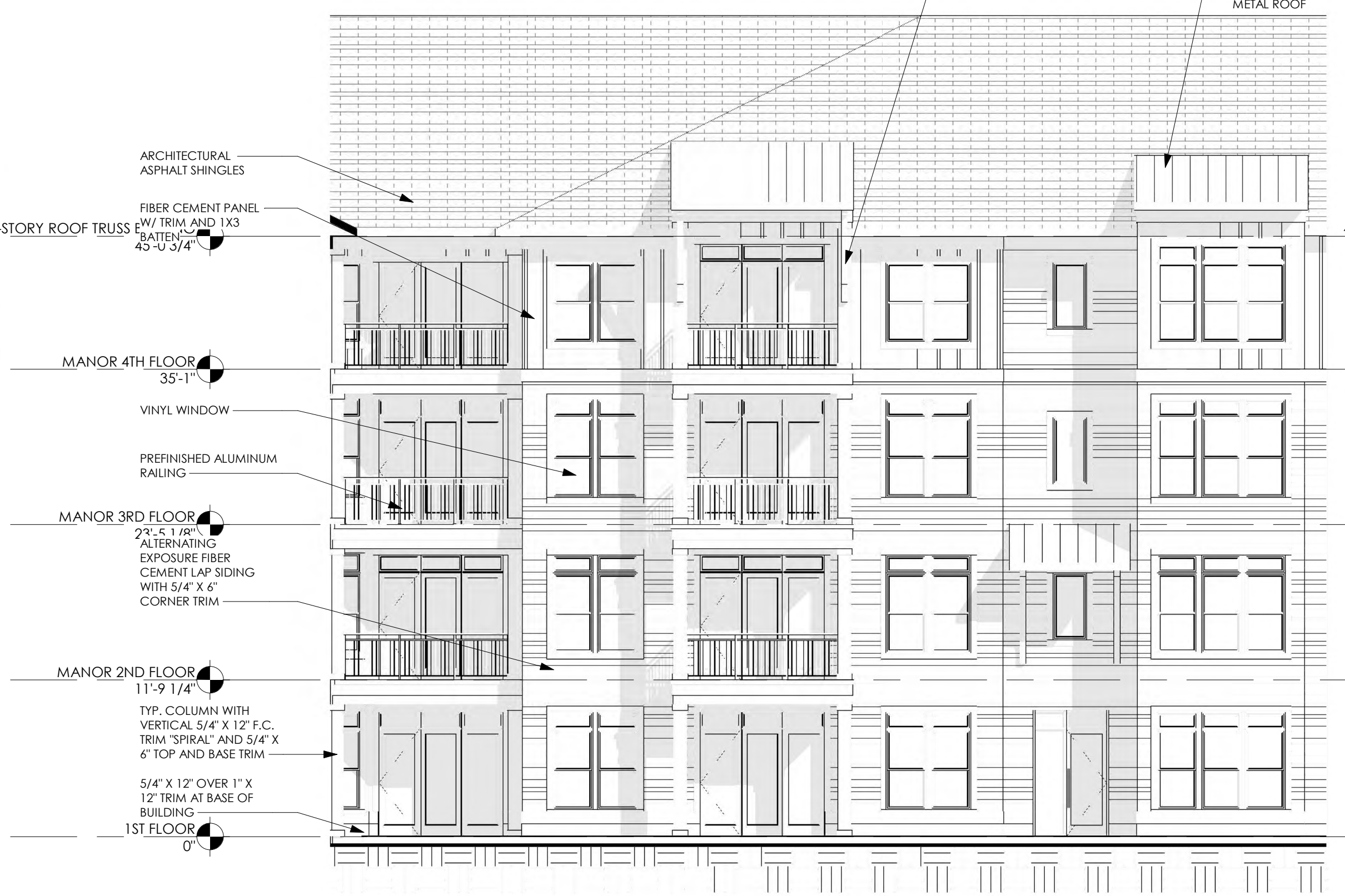
2 BLDG TYPE A - REAR ELEVATION 2 1/8" = 1'-0"
