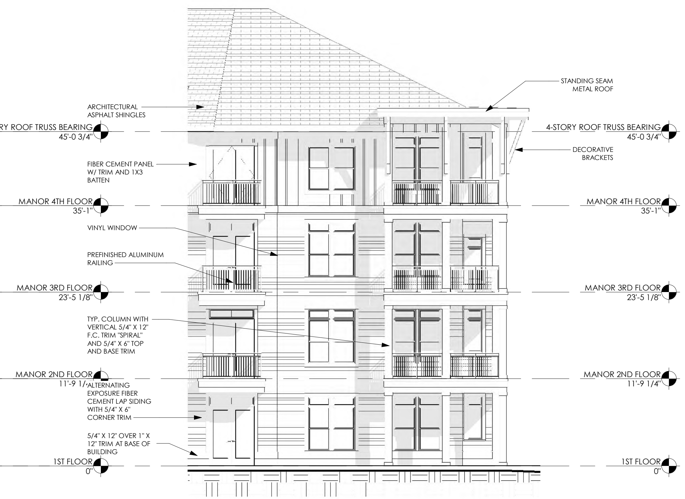
1 BLDG TYPE A - REAR ELEVATION 1 1/8" = 1'-0"
