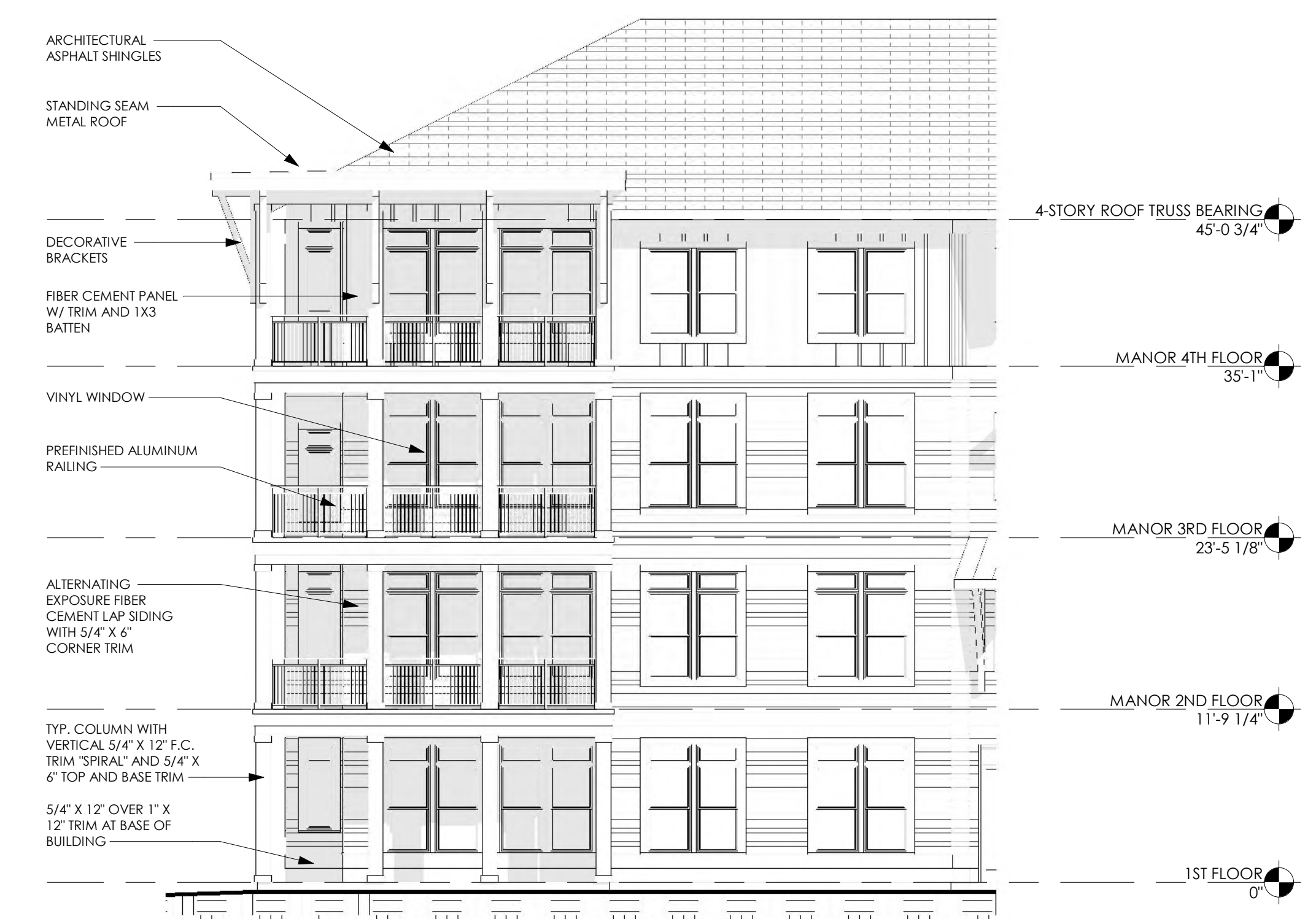
3 BLDG TYPE A - FRONT ELEVATION 3 1/8" = 1'-0"
