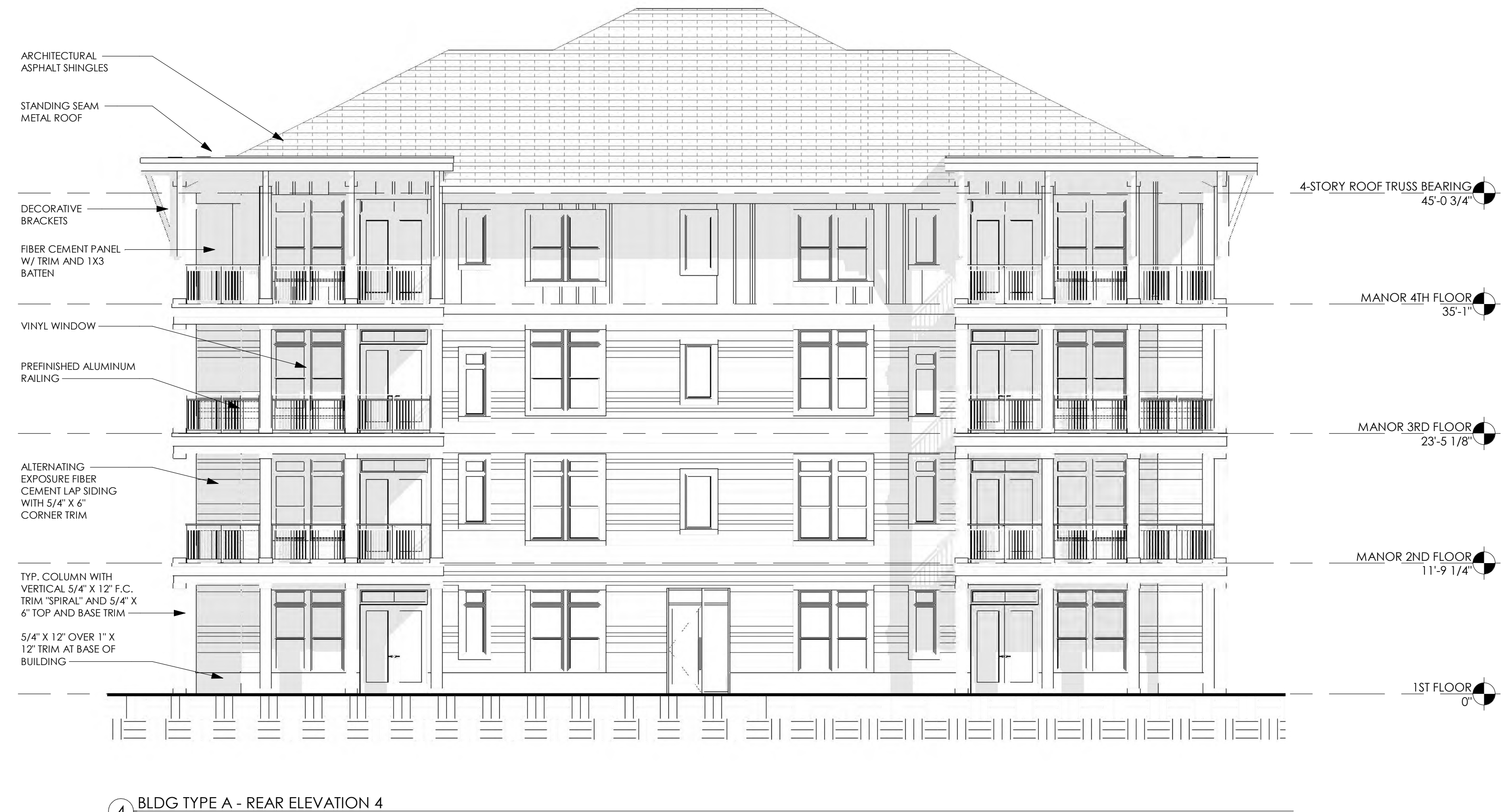
4 BLDG TYPE A - REAR ELEVATION 4 1/8" = 1'-0"
