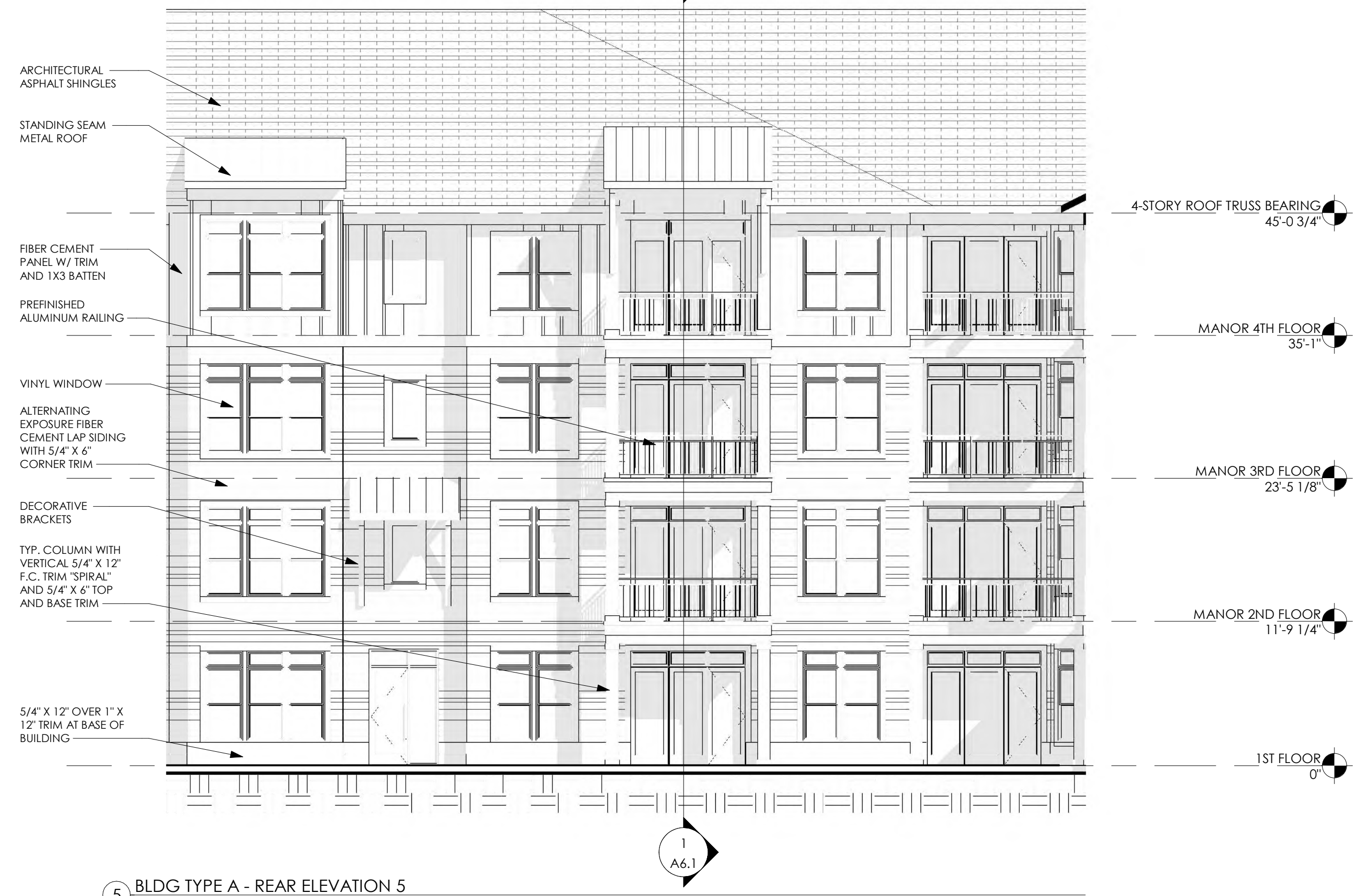
5 BLDG TYPE A - REAR ELEVATION 5 1/8" = 1'-0"
