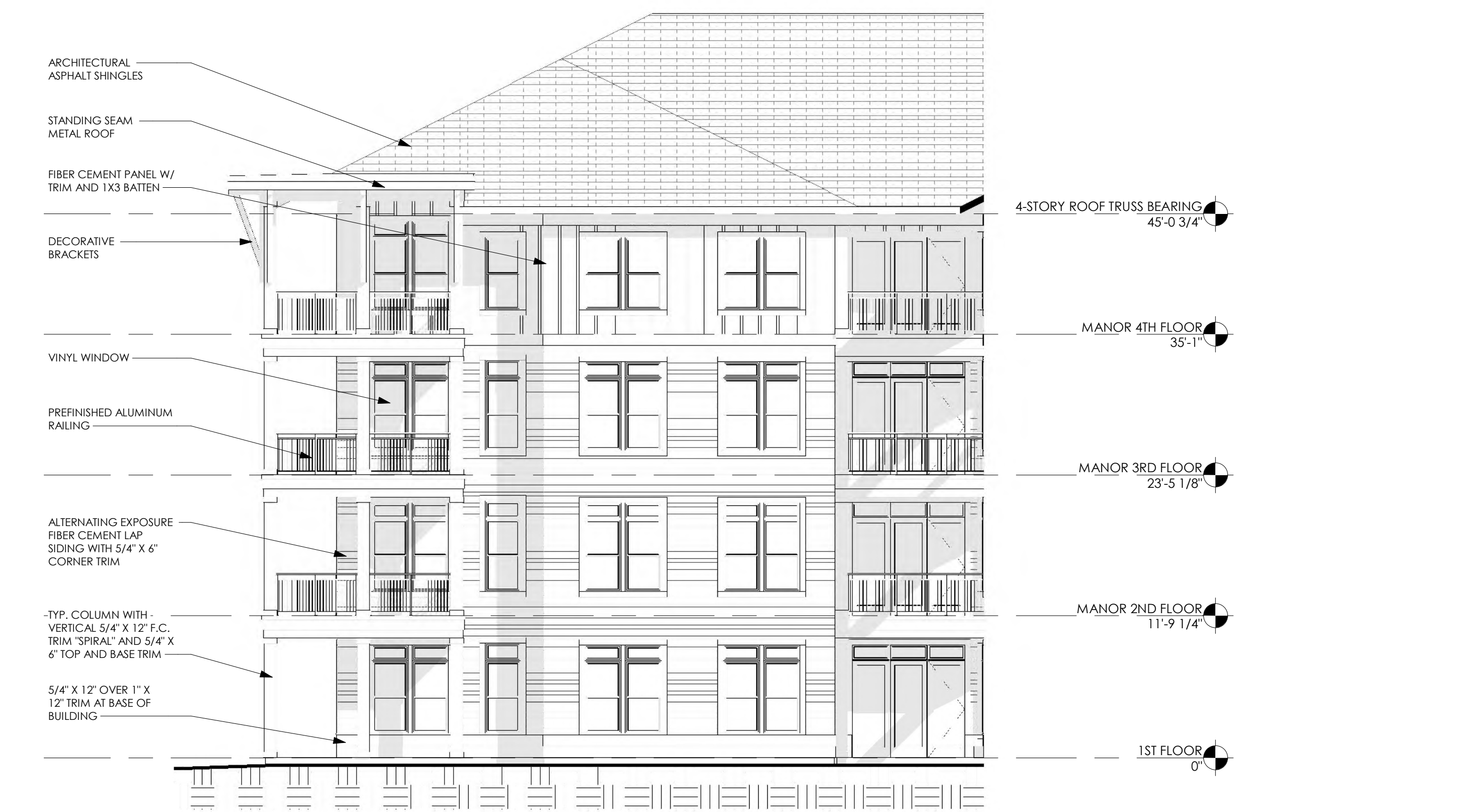
③ BLDG TYPE A - SIDE 2 ELEVATION 1 1/8" = 1'-0"
